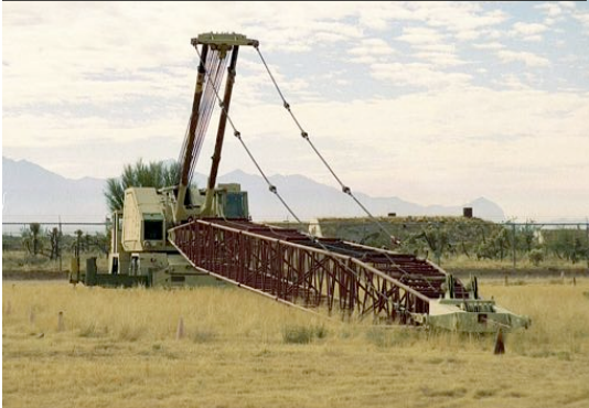
The top photograph shows the crane that was initially used to destroy 365 B-52s. The bottom photograph shows just how effective the crane and guillotine were.
