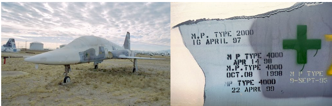
The photograph to the left shows a Northrop T-38 Talon covered with white Spraylat. The photograph to the right shows a blow-up of the fuselage with the safety and type storage markings. The green cross means that the canopy and ejection seat explosives were removed September 9, 1995. It also means that fuel, oil and hydraulic fluids were drained at the same time and that their systems were coated with an oil preservative. The type storage markers indicate that the aircraft entered type 2000 storage in April of 1997 and type 4000 storage in April of 1998. Lastly, the markings also show that the aircraft was reconfirmed for type 4000 storage in April of 1999. Regrettably, because this aircraft has been relegated to being a parts supplier to others in the field, it will most likely never fly again and end up as just salvage.
